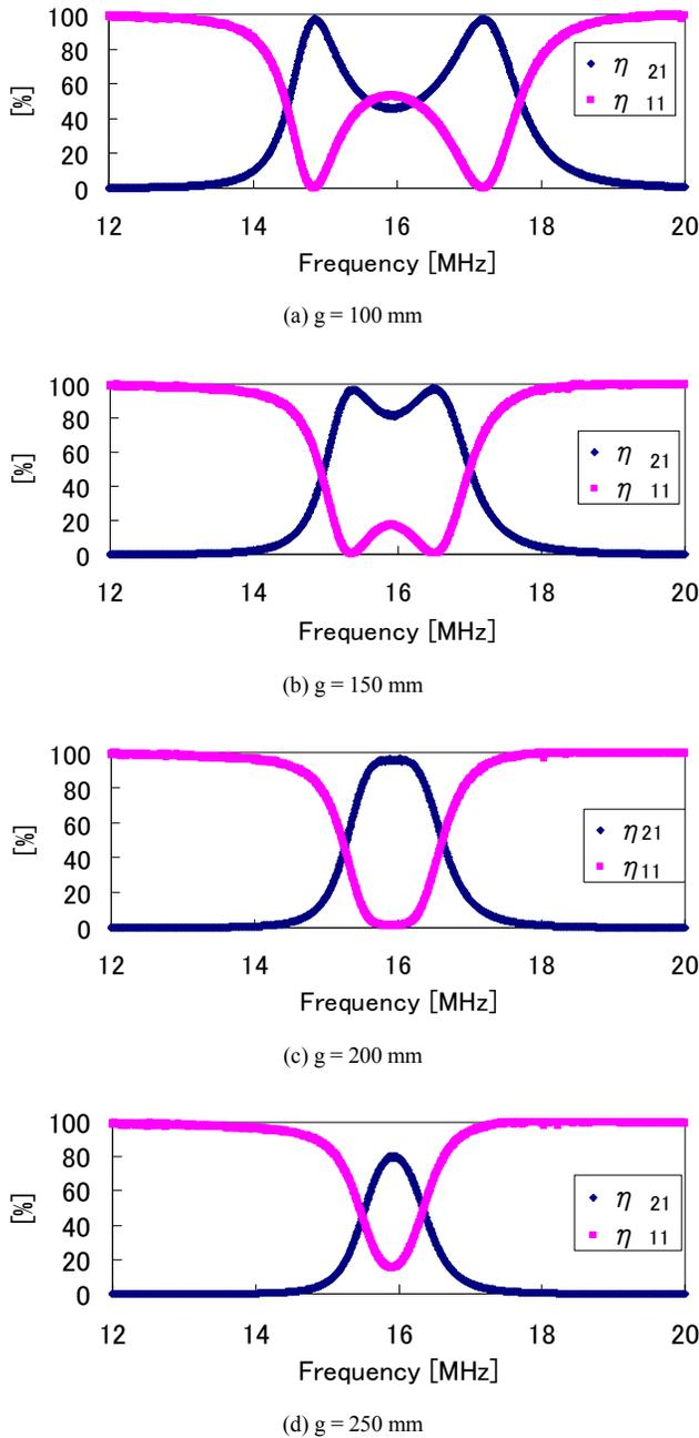
Fig. 6 Experimental results of efficiency in each gap
