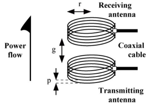
Fig. 4 Parameters of antennas
