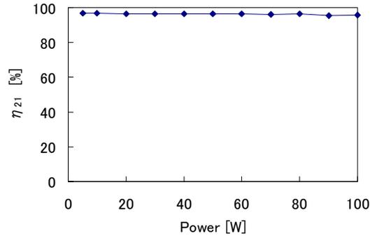
Fig. 12 Power vs. efficiency in high power
