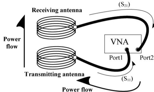
Fig. 5 Experimental setup for low power
