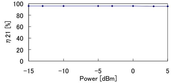
Fig. 11 Power vs. efficiency in low power
