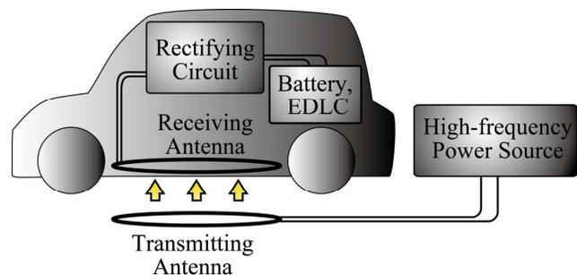
Fig. 1 Concept of contactless power transfer system for EV
