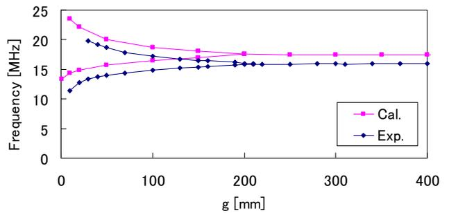
Fig. 8 Air gaps  $g$  vs. two resonant frequencies  $f_m$  and  $f_e$  ( $f_m < f_e$ )
