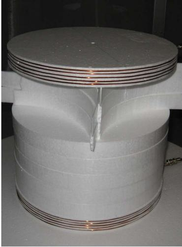
Fig. 2 Transmitting antenna and Receiving antenna
