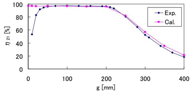
Fig. 7 Air gaps  $g$  vs. efficiency of power transfer  $\eta_{21}$
