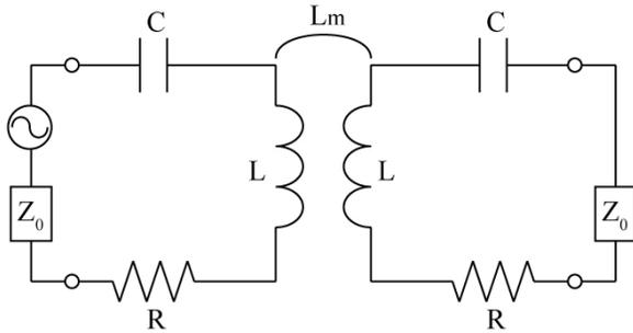
Fig. 10 Equivalent circuit of magnetic resonant coupling
