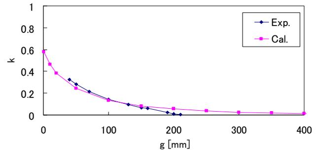
Fig. 9 Air gaps  $g$  vs. coupling coefficient  $k$
